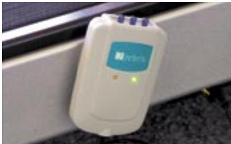
The infrared synchronization adapter is connected to the junction box of the treadmill ergometer.
