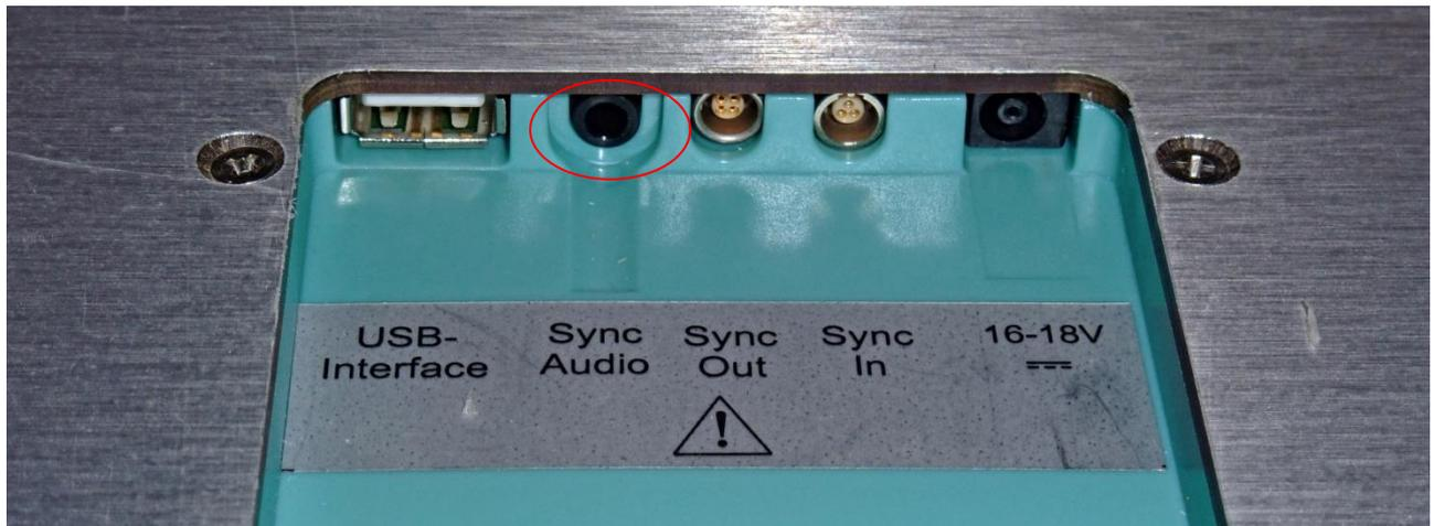
The synchronization is effected by imprinting a tact signal on the soundtrack of the video recording. This data is evaluated automatically by the application software WinFDM for synchronizing the platform data and the video signal.
