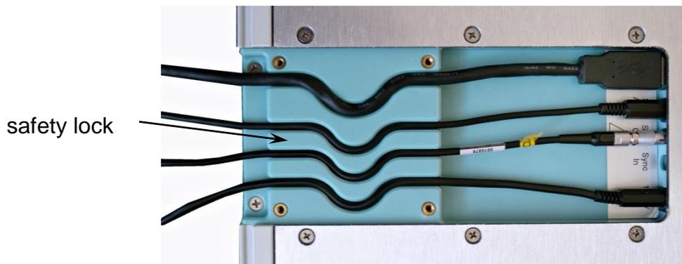
If the power supply unit and the USB cable are connected to the sockets of the platform, please close the lid of the safety lock and fasten it to the housing by means of the four screws supplied with the platform.
